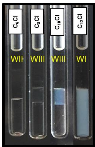
Figure 7. Oil scan performed for 3% C 9 -tetraol/1-Chloro-alkane/Water systems after 2 days equilibration period at 75°C.
